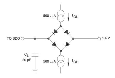
IGURE 3. Load circuit for digital interface timing.
